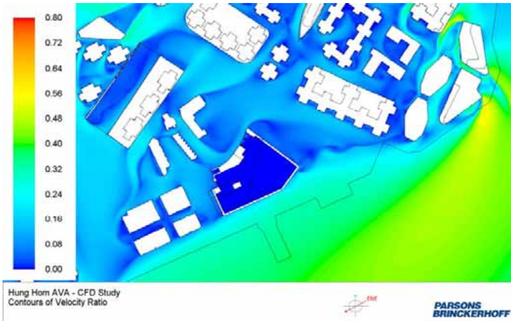
Velocity Ratio Plot at 2m above Ground for East-North-Eastern Wind - Notional Scheme
