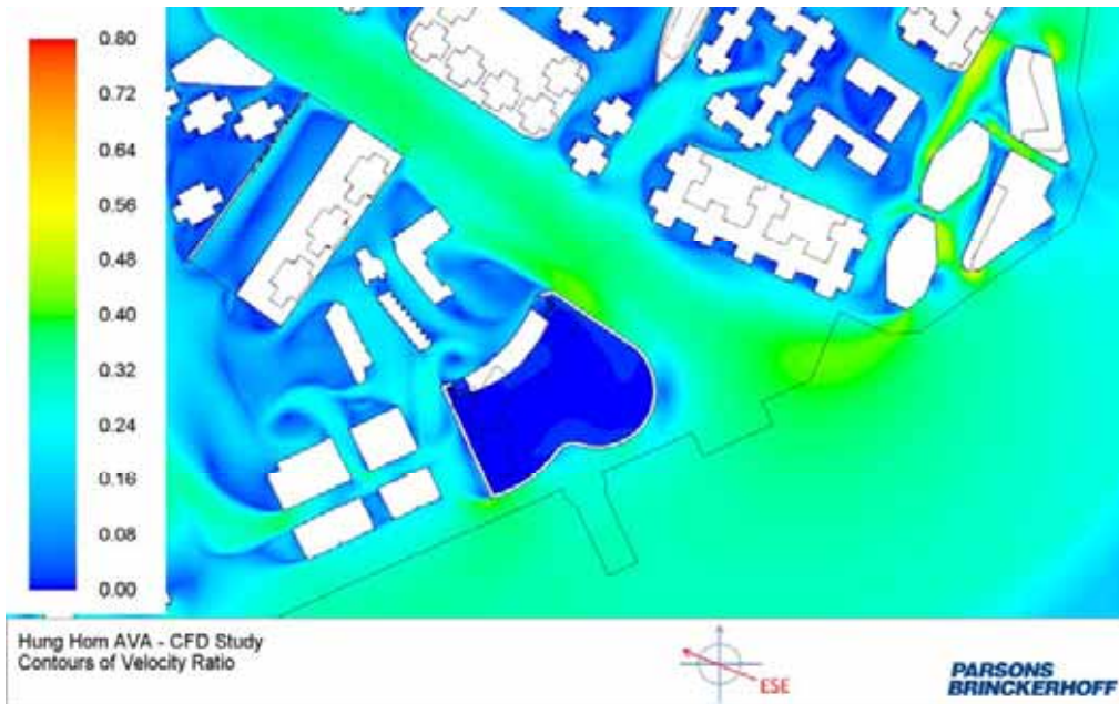
Velocity Ratio Plot at 2m above Ground for East-Southeastern Wind - Urbis Scheme
