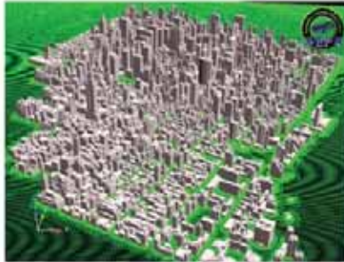
An example of the detailed building geometry for Manhattan, presented with a surface mesh on the ground; the mesh was created using Harpoon from CEI
