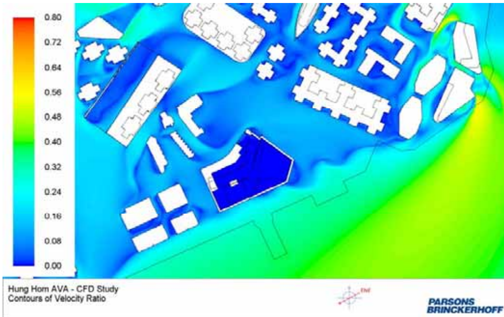
Velocity Ratio Plot at 2m above Ground for East-North-Eastern Wind - Proposed Scheme
