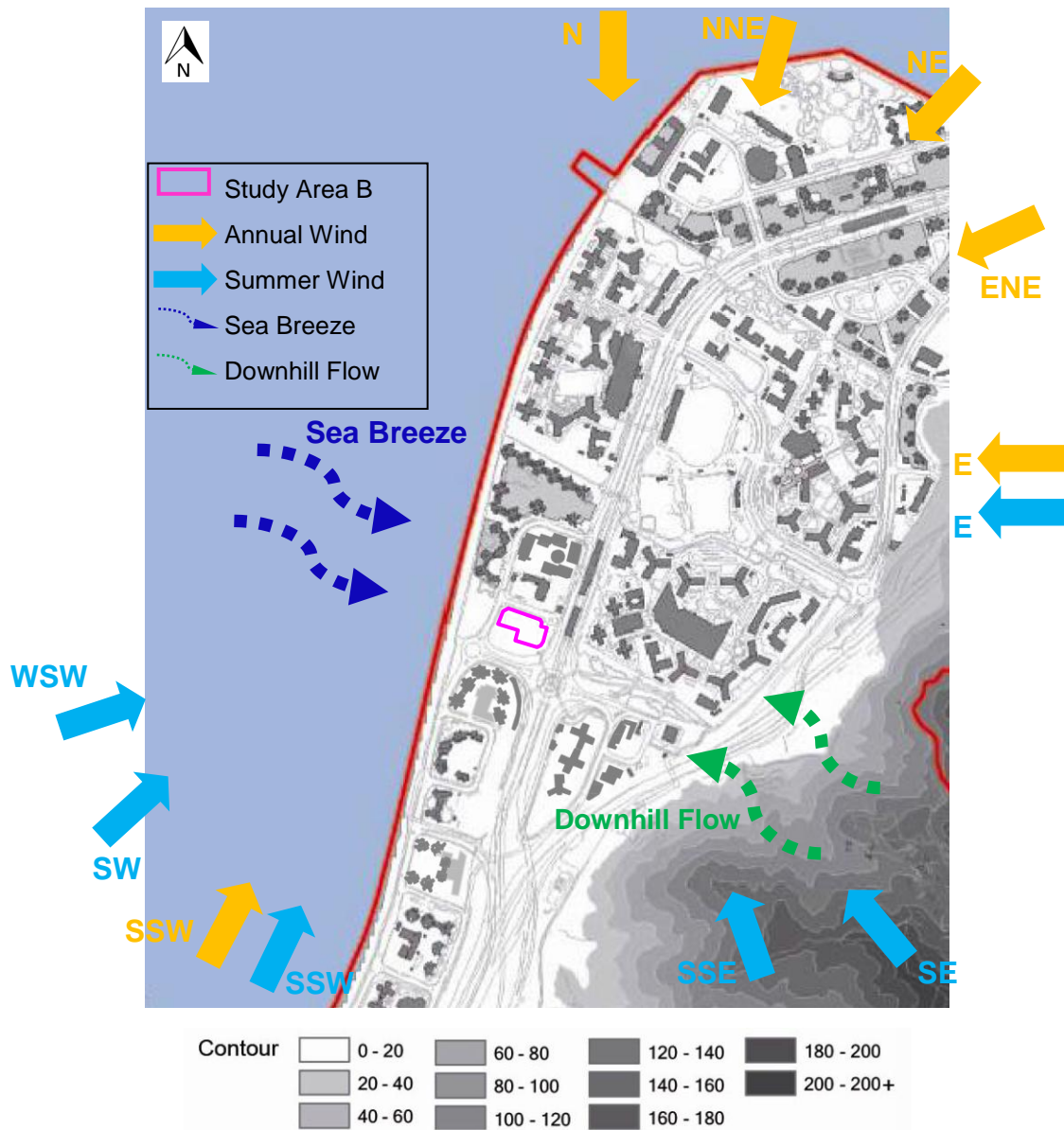
Figure 3.4 Digital Elevation Map and natural air movement around the Study Area B
