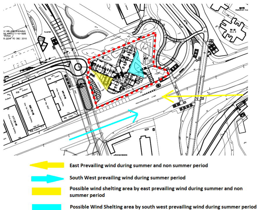
Figure 11 Potential Wind Sheltering by Project of Summer E & SW and non-Summer E Wind Penetration
