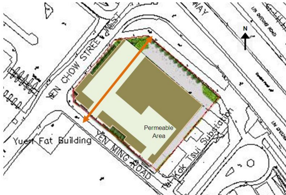
Figure 5-3 Permeable Design at G/F (at 5.1 mPD) Workshop with Wind Flow (Orange Line)
