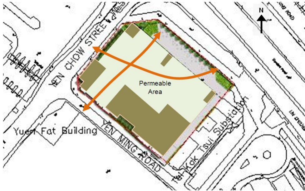
Figure 5-5 Permeable Design at 2/F (at 20.0 mPD) Carpark with Wind Flow (Orange Line)
