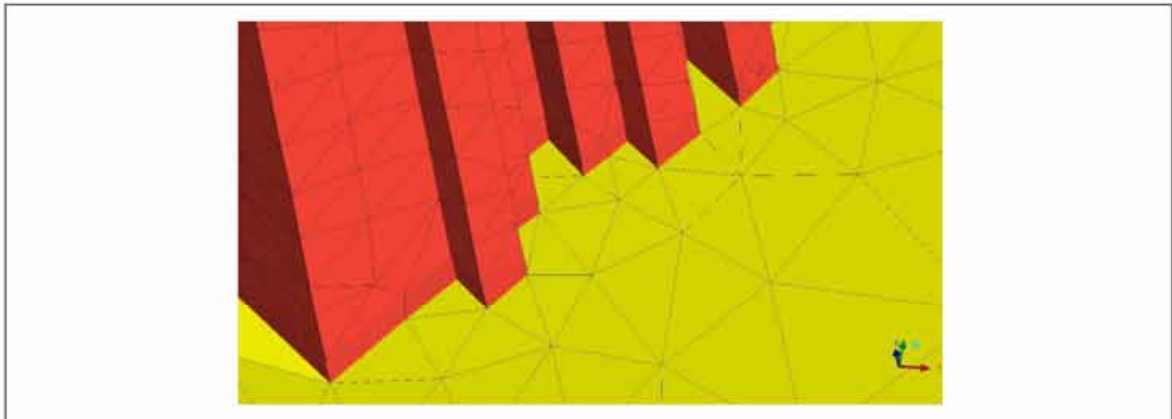
Figure 3.4(b) 4 layers of Prism Mesh Cells Setup in the CFD Model
