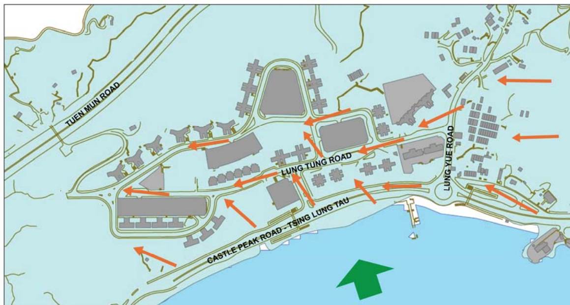
Figure 5.6 Summer prevailing wind directions of Tsing Lung Tau area (orange arrows). In addition, the area also benefits with the sea breezes from the south (green arrow).
