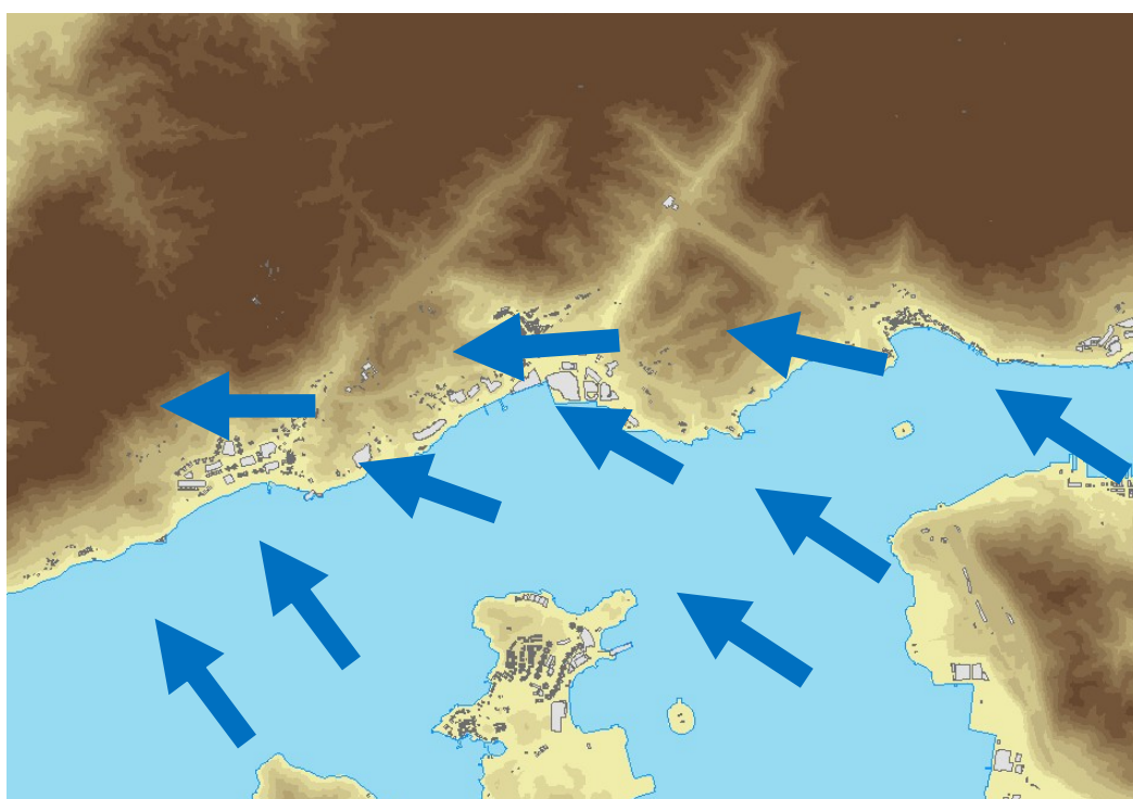
Figure 3.17 Prevailing wind directions at 60m (summer months Jun-Aug) based on MM5-CALMET model simulation.
