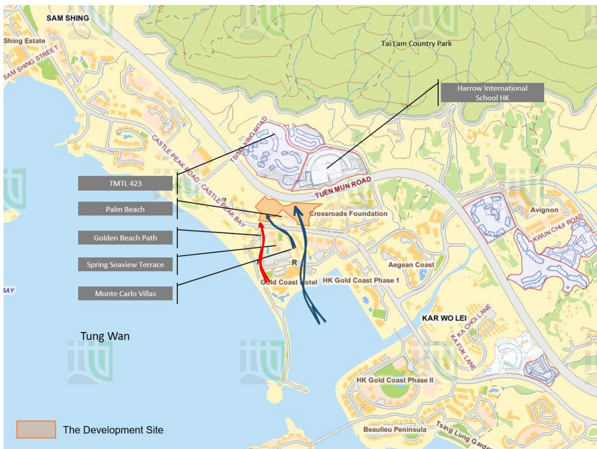
Figure 10 Major air paths under SSE wind
