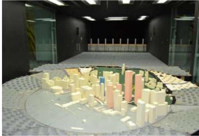
Figure 7 Wind tunnel model and setup, viewed from Northwest
