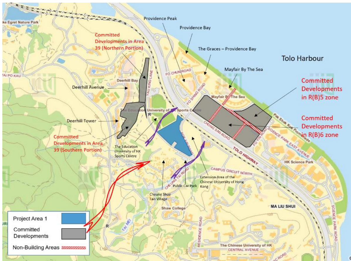
Figure 11 Major air paths under SW and SSW winds with the presence of notional development at Project Area 1
