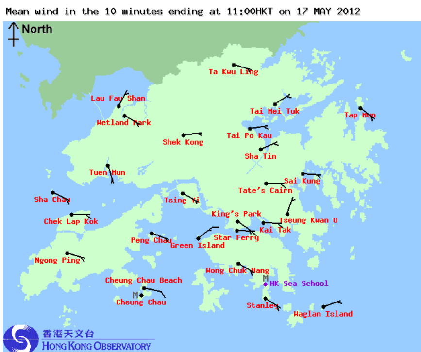
Figure 3.1 Some of the HKO stations in Hong Kong. This is a screen capture at 11am on 17 May 2012 from the HKO website. The arrows show the wind directions and speeds of the time.
