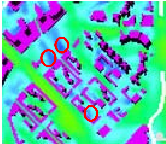
Figure 26 Stagnant zones in a typical courtyard
